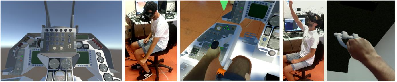
Fig. 3. From left: user view of the XR-Cockpit as seen in VR mode; external views of a user performing two tasks on the cockpit and the corresponding user views in MR mode (cropped)
