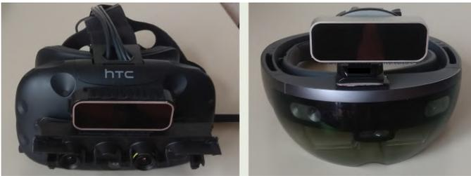
Fig. 4. The two headsets used for our tests. Left: HTC Vive with Leap Motion and Zed Mini camera. Right: Microsoft HoloLens with Leap Motion.
