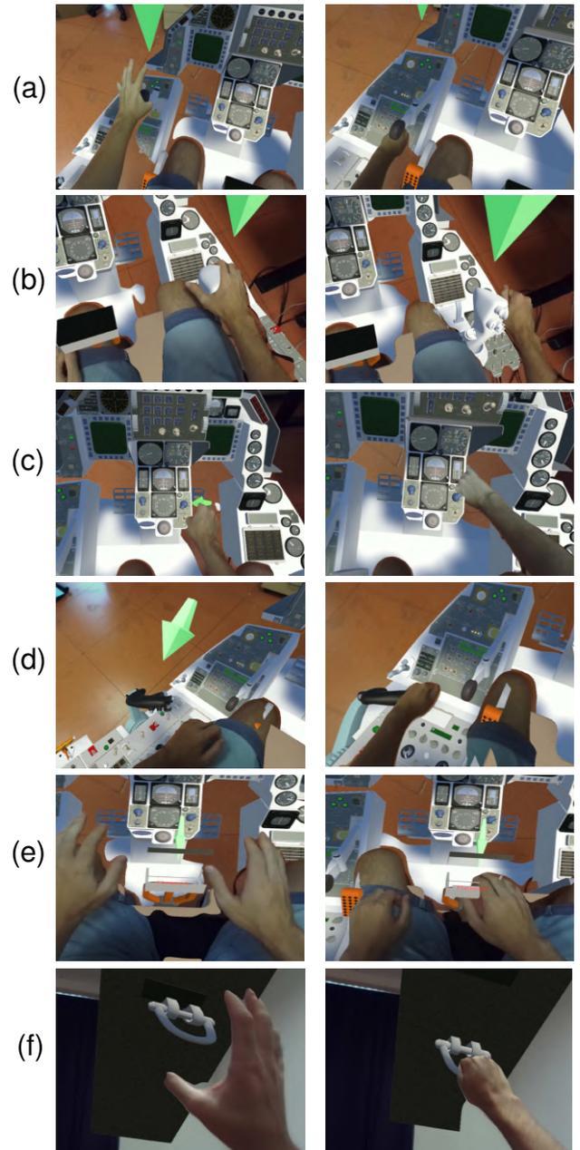
Fig. 2. Virtual manipulations of the six interactive virtual tools as seen by users in video see through Mixed Reality. (a) Left lever. (b) Joystick. (c) Knob. (d) Bottom lever. (e) Box with button inside. (f) Handle.
